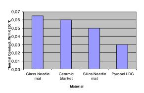
.PYROPEL LDG is a non-fabric 100% flexible PI with a new super-insulating gel, and lined on one side with a silicon coated glass fabric, studied for industrial applications where flexibility and high thermal insulation up to 333°C are required. Unlike traditional fibers, PYROPEL LDG is ecologic, easy to mold and without organic and inorganic bonders. Up to 280°C, PYROPEL LDG guarantees strong energy savings. Also available matched with ECA 300 aluminized cloth
